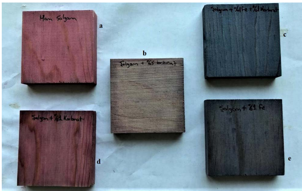
Figure 1. Dyed red pine samples. a is raw turnip juice, b is turnip juice +5 g/L NaHCO 3 , c is turnip juice +1 g/L FeSO 4 .7H 2 O +1 g/L NaHCO 3 , d is turnip juice +1 g/L NaHCO 3 , e is turnip juice +1 g/L FeSO 4
