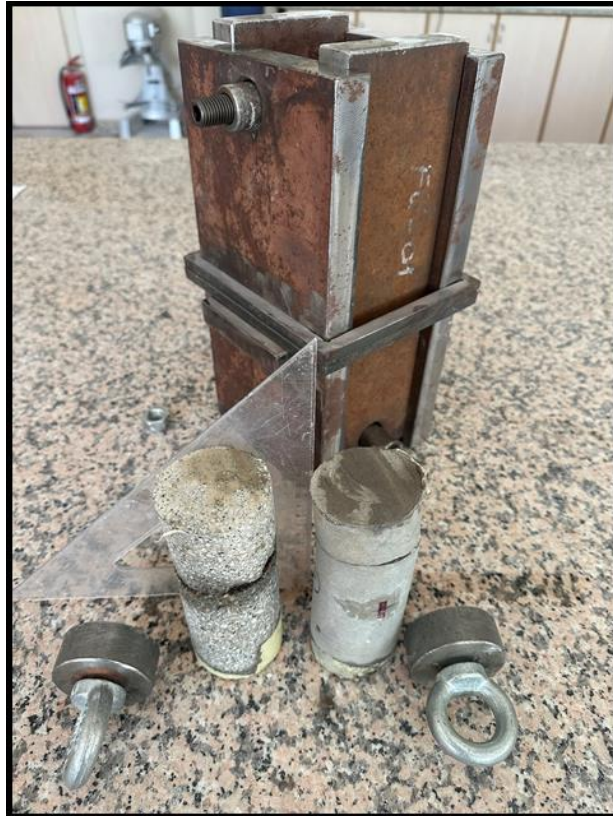
Figure The apparatus used for the direct tensile test, the grips utilized, and the failed samples.
