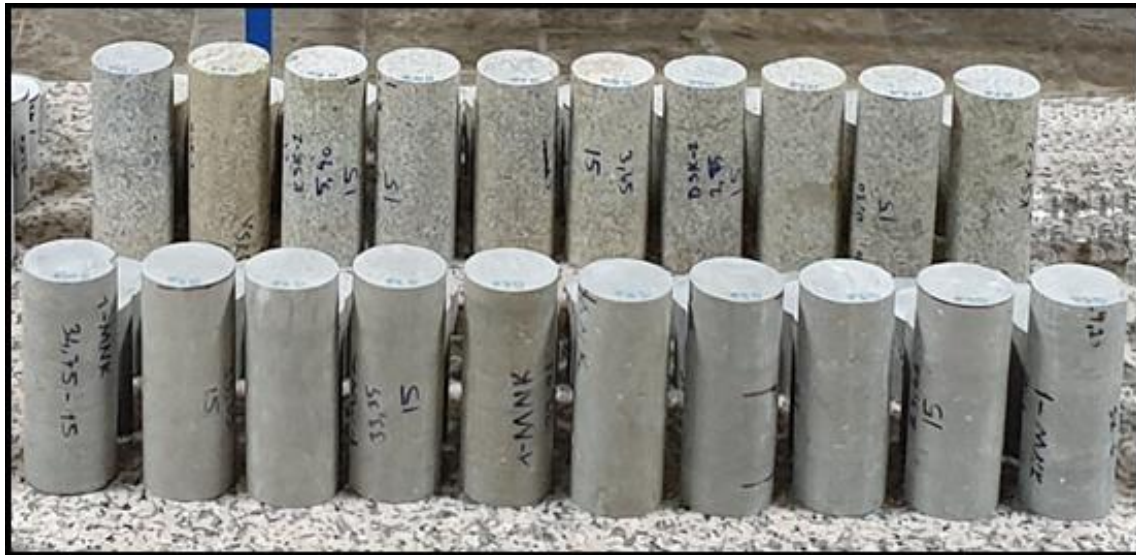
Figure 3 The specimens used for the direct tensile strength test
