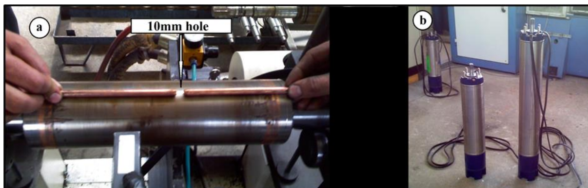
Figure 3. Photographs of the faulty rotor; a- Broken bar fault, b-Motors used
