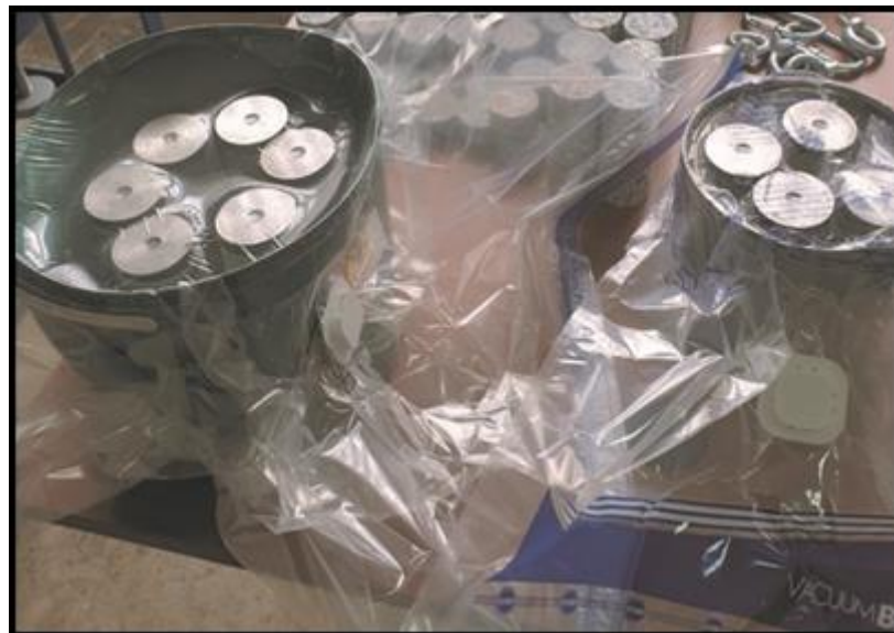
Figure 4 Curing phase of the specimens
