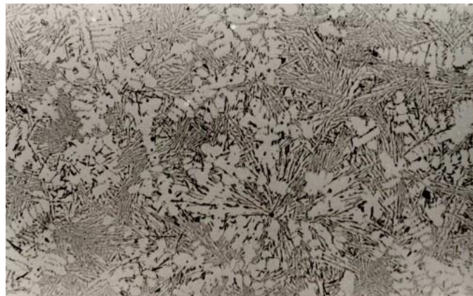
Figure 3 Microstructure of Al 0.7wt % Si 0.02wt % Sr alloy
