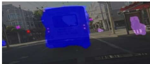
Figure 11. Red indicates red light, dark purple indicates traffic signs, magenta indicates pedestrians and blue indicates dynamic objects.
