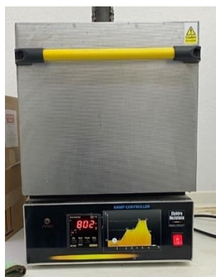
Figure 2. Muffle furnace used in the production of activated carbon
