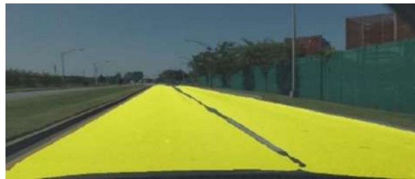
Figure 4. Visualization of the drivable area segmentation result. Each lane is separated in terms of drivable area.
