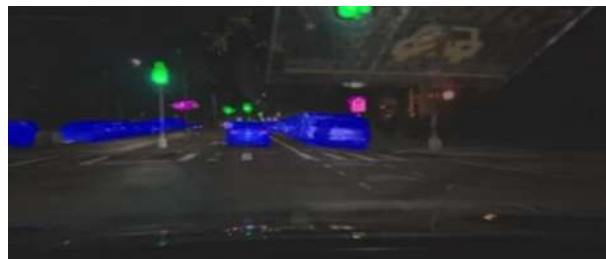
Figure 10. Green indicates green light, dark purple indicates traffic signs and blue indicates dynamic objects.
