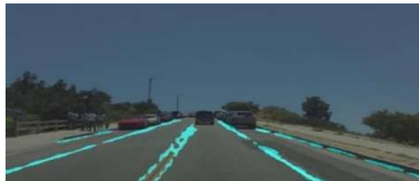
Figure 6. Visualization of the lane line detection result. Road curbs and lane lines are detected. These are the direct masks from predictions and are not post processed by any means of line fitting.
