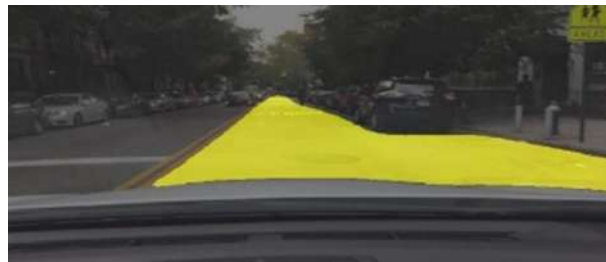
Figure 3. Visualization of the drivable area segmentation result. In two-way road case, incoming lane is not segmented.
