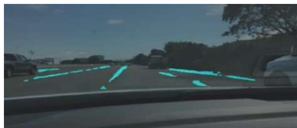
Figure 7. Visualization of the lane line detection result. Dashed lines are detected.
