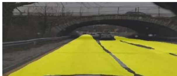
Figure 5. Another visualization of the drivable area segmentation results that shows each lane is separated in terms of drivable area.
