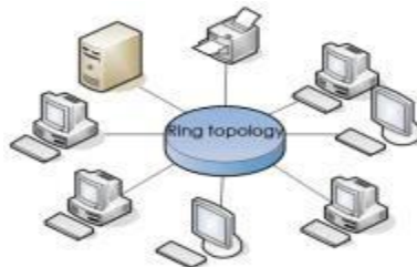
Figure 6: Ring Topology Source: Keçeli, 2011
