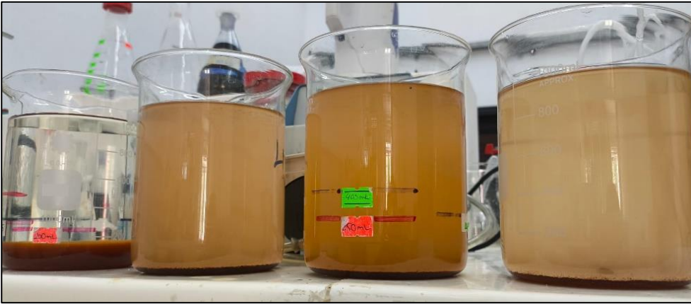
Figure 2. Settling behavior of the materials after the P removal tests (Samples in the beakers from left to right: LDH w , LDH 50 , LDH 75 , LDH 105 )
