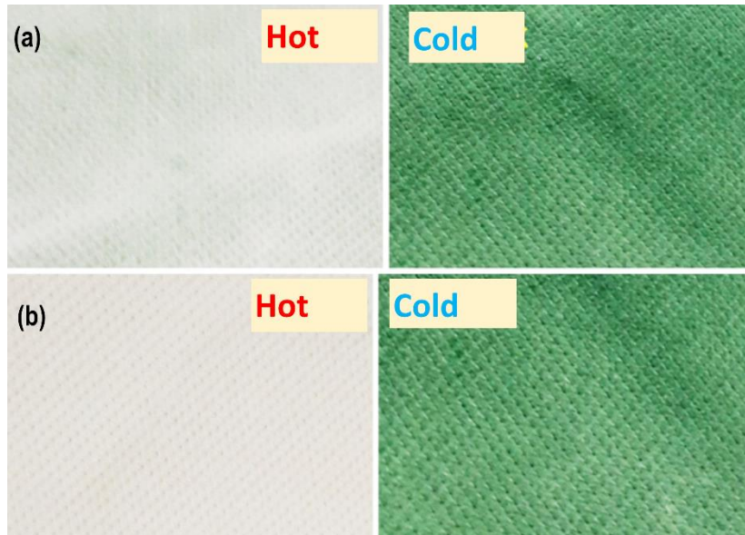
Figure 3. Photographic images of fabrics taken in heat and cold (a: Fabric 1 treated with a nanocapsule bath containing zinc oxide (ZnO) particles b: Fabric 2 treated with a nanocapsule bath without the inclusion of ZnO particles)
