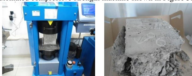
Figure 3.1.1: Compressive strength machine
