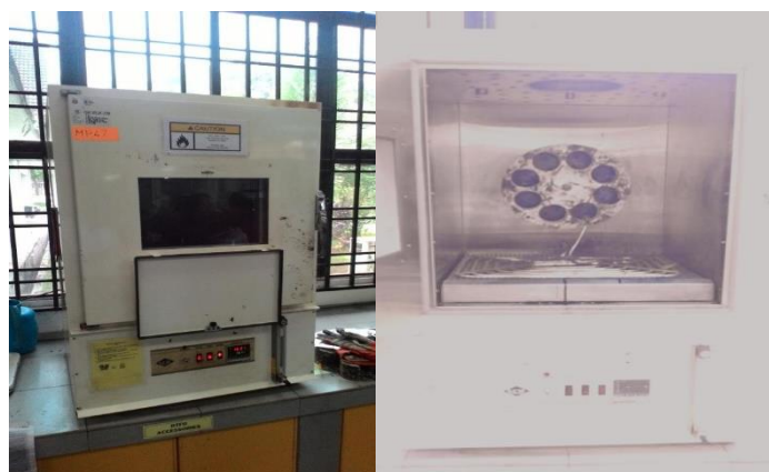
Figure 3.4 Rolling Thin Film Oven Test ( RTFOT) machine
