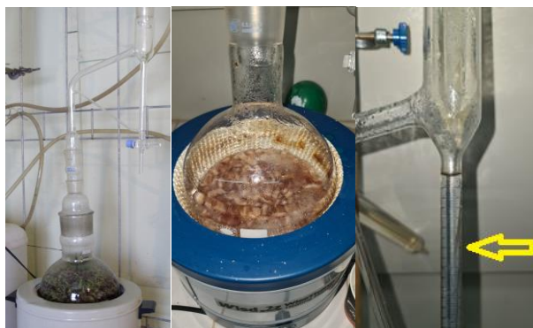
Figure 1. Stages of obtaining aromatic water in Clevenger device. Yellow arrow points to aromatic water.
