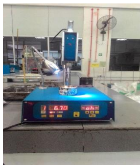
Figure 3.2 Penetration test setup
