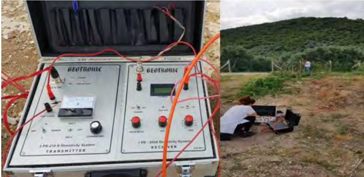
Figure 4. Views from electrical resistivity device and GNSS measurements on the installed profile.
