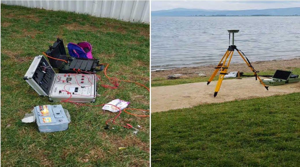
Figure 4. ERT and GNSS measurements performed near St. Neophytos Basilica.
