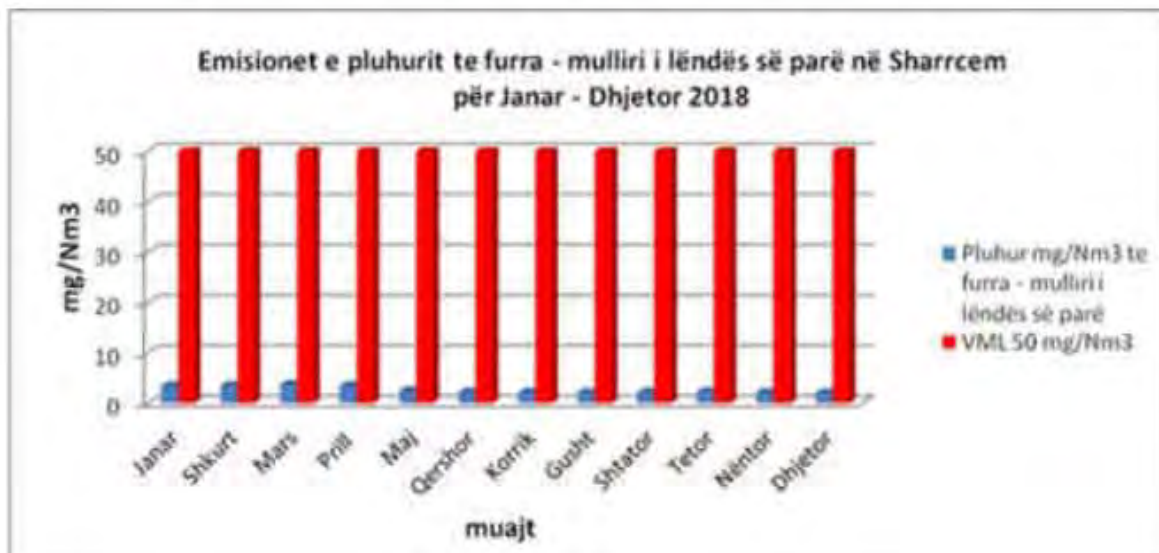
Fig.8. Average monthly value of dust emissions in the furnace - raw material mill at mg / Nm3 / 2018.
