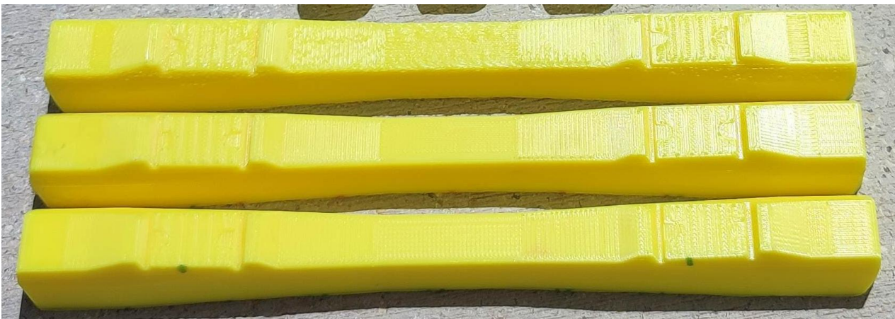
Figure 2. Miniature 3D-printed B70-type railway sleeper models fabricated at different flow rates (from top to bottom: 1.050, 0.960, and 0.926)
