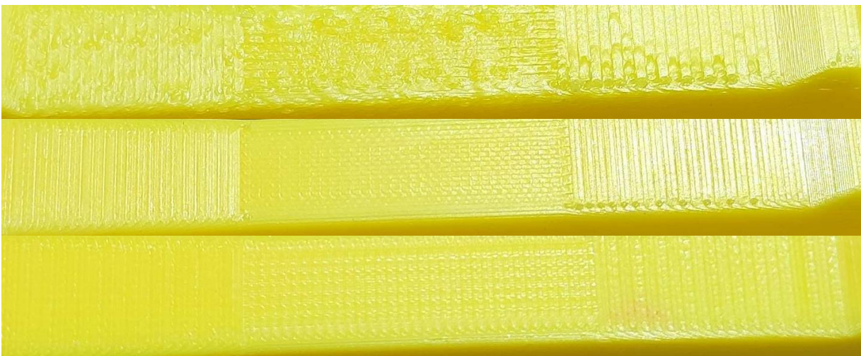
Figure 3. Zoomed-in views of the miniature 3D-printed B70-type railway sleeper models (flow rates from top to bottom: 1.050, 0.960, and 0.926)
