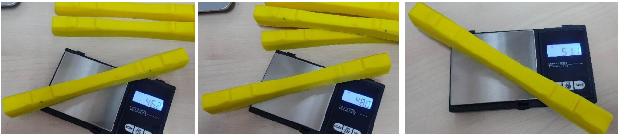
Figure 4. Miniature B70-type sleeper models being weighed on a precision scale, showing weight readings for flow rates of 0.926, 0.960, and 1.050 (left to right)
