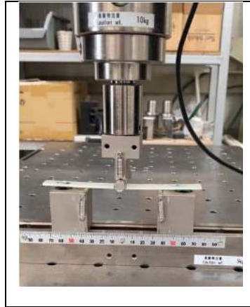
Figure 5: The support span. 3-point bending test was done at 1mm/min. at Shimadzu AGS-X series test device
