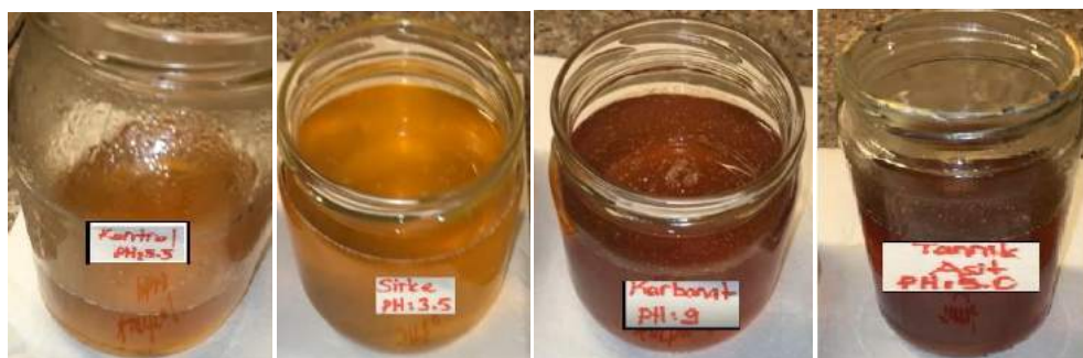
Figure 2. The arranged dye solutions for sun dyeing: a) control with pH 5.5, b) pH 3.5 by vinegar, c) pH 9.0 by carbonate and d) pH 5.0 by tannic acid
