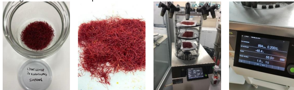
Figure 12-13-14-15. Drying saffron samples by procedure using Lyophilization
