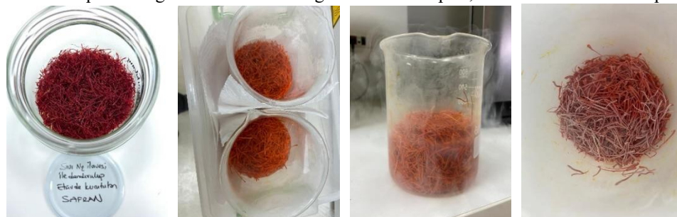
Figure 8-9-10-11. Dehydration procedure using liquid nitrogen drying saffron samples
