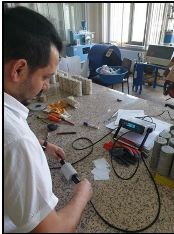
Figure 2. Sonic wave velocity testing
