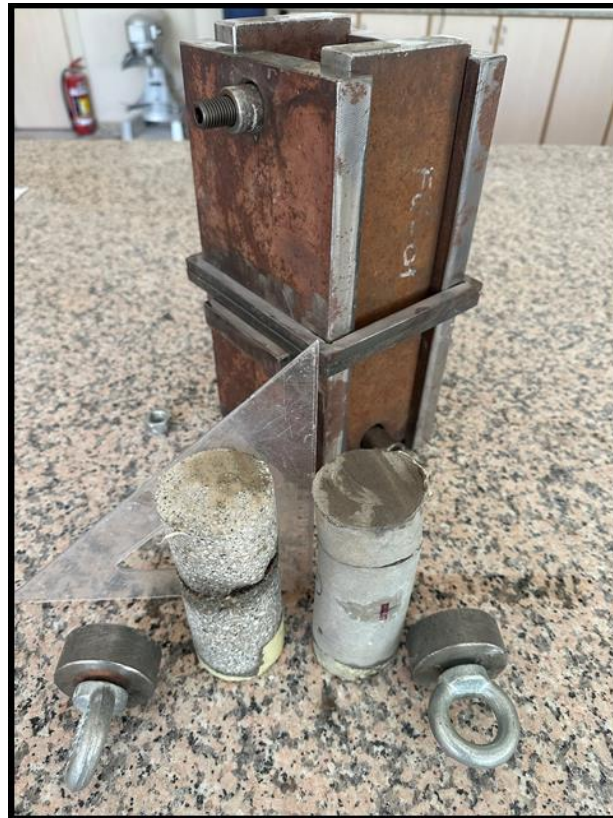
Figure 5. The apparatus used for the direct tensile test, the grips utilized, and the failed samples.
