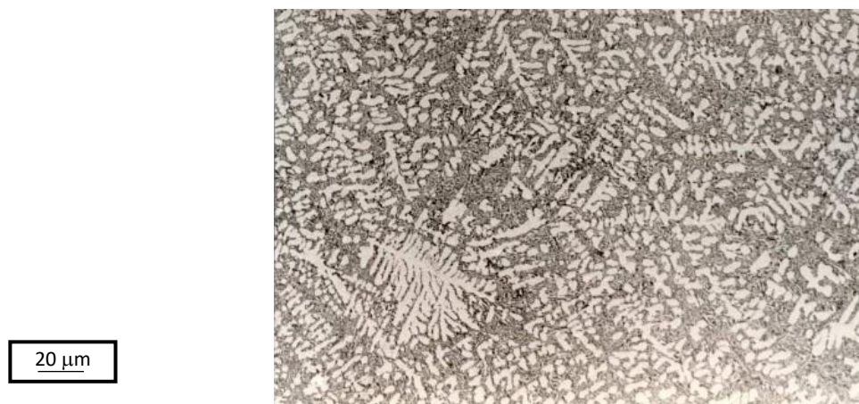
Figure 2. Microstructure of Al-10.7wt%Si-0.02wt%Sr alloy
