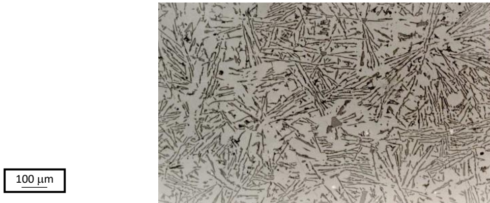
Figure 1. Microstructure of Al-10.7wt%Si (unmodified) alloy
