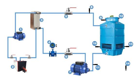
**Figure 1.** Experimental setup. 1: Boiler line water pump, 2:Gas fired hot water boiler, 3: Plate heat exchanger, 4: Flowmeter, 5-6: Flow control valve, 7: Cooling tower water pump, 8-9-11-14:Thermocouples, 12: Cooling tower, 10-13:Wet bulb temperature measuring devices.
