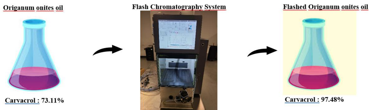
Figure 5. Purifying Carvacrol Compound By Using Flash Chromatography
